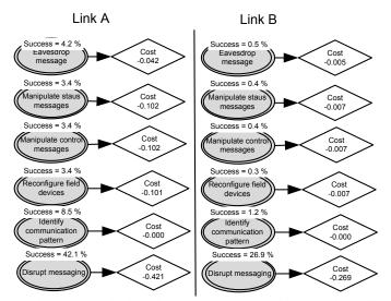
Figure 3 – Results from the security assessment of link A and B. Ellipses show the attack goals and the probability that they can be reached; rhomb shaped utility nodes display the expected losses associated with each attack attempt.
