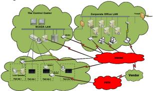
Figure 2. There are often many different communication interfaces to the SCADA system which are not depicted in the architectural model.
