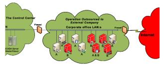
Figure 1. During the authors' practical security assessments at one facility "A" we identified that its corporate office LAN was closely interconnected with another company "B". The separation from other organizations was more or less chimaeras due to awful configurations and badly chosen passwords on critical part of the infrastructure equipment maintained by the outsourcing partner.
