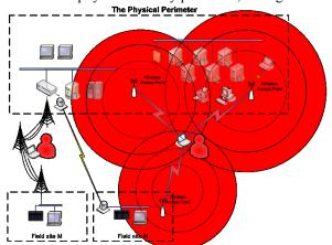
Figure 4. The use of wireless technologies easily extends the logical access perimeters beyond the physical security perimeter.
