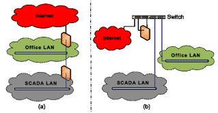
Figure 3. Logical and physical mismatch. In the logical schema to the left (a) one gets the impression that the different networks are well separated. However, in reality it looks like (b) the networks are physically connected to the same switch and the separation is only made logically by the VLAN configuration.
