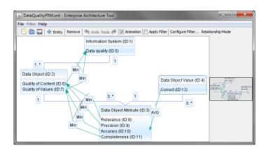
Fig. 4. The PRM for data quality analysis showing classes and attributes relevant for the analysis.
